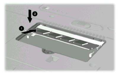
Inserting a memory expansion module
